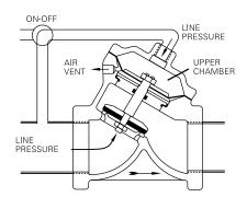
Drip-Tight Closing: Closure is obtained by directing line pressure or equivalent independent pressure into the upper chamber. This pressure on the large diaphragm area causes the valve disc to seal against the seat.
