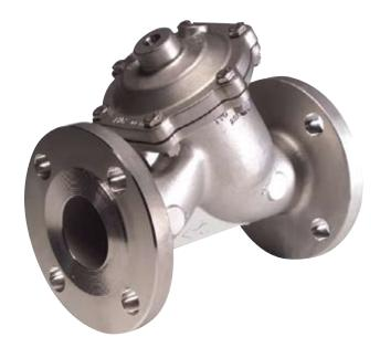
The AquaMatic V46 Series Stainless Steel Valves are designed to permit higher flow rates than similar-sized diaphragm-operated valves. They are available in 1-, 1-1/2- and 2-inch diameters in threaded or flanged ends. With all stainless steel internals and no internal threads, the V46 is ideally suited for corrosion-resistant applications.
